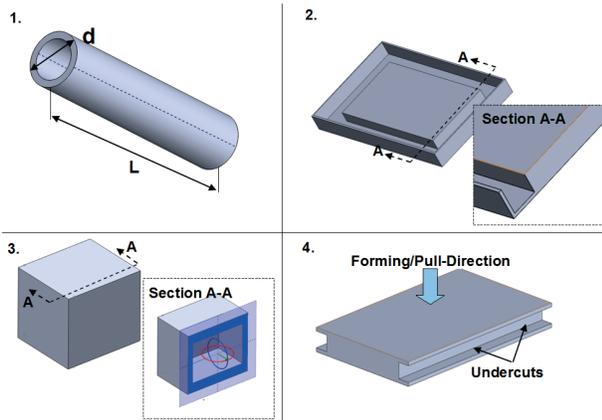
Figure 2. Design features not suited for compression molding
