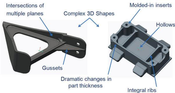
Figure 1. Design features well suited for compression molding
