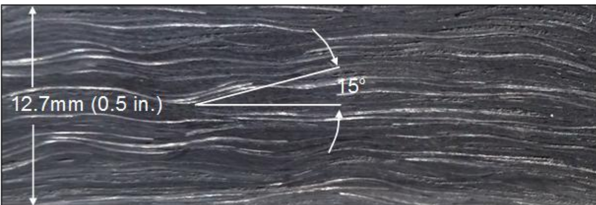
Figure 3. Stacking of BMC through-the-thickness (photograph of unpolished specimen).
