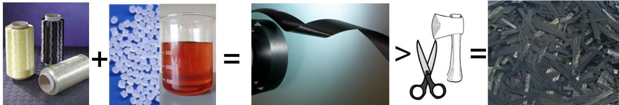
Figure 2. Bulk Molding Compound Preparation
