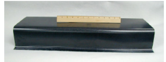
Demonstration part of 100+ ply of TC275-1, less than 1% voids.
